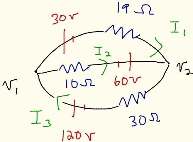
" $\Omega$ " = Ohms, " $\text{V}$ " = volts
